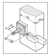
Because the B dimension is less than 100 mm, install a spacer under the post fitting. This means that the B dimension is 100 mm.
