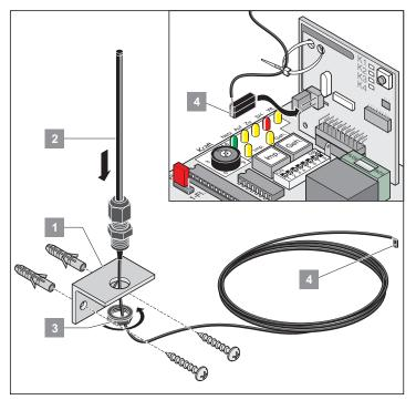
Connect external antenna to connection.
